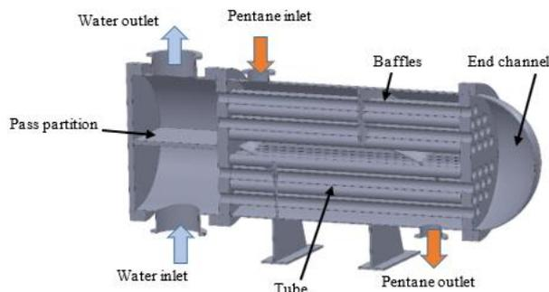
**Fig. 12.** Transverse cross-sectional model of the HTX.
