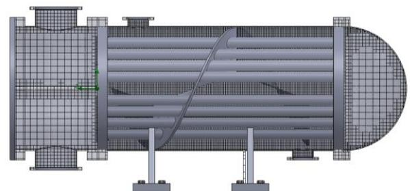
Fig. 9. Meshing illustration of shell and tube HTX.
