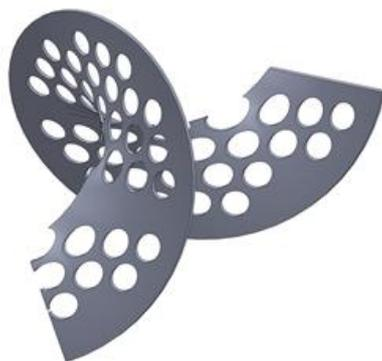
**Fig. 13.** Incontinence pads Screw (Helical Baffle).
