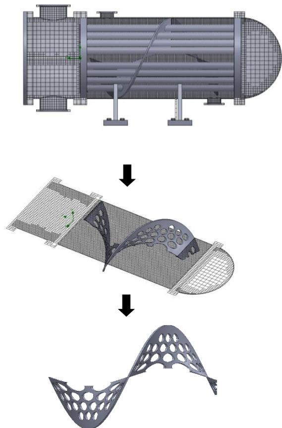
Fig. 4. The geometry and generated grid.
